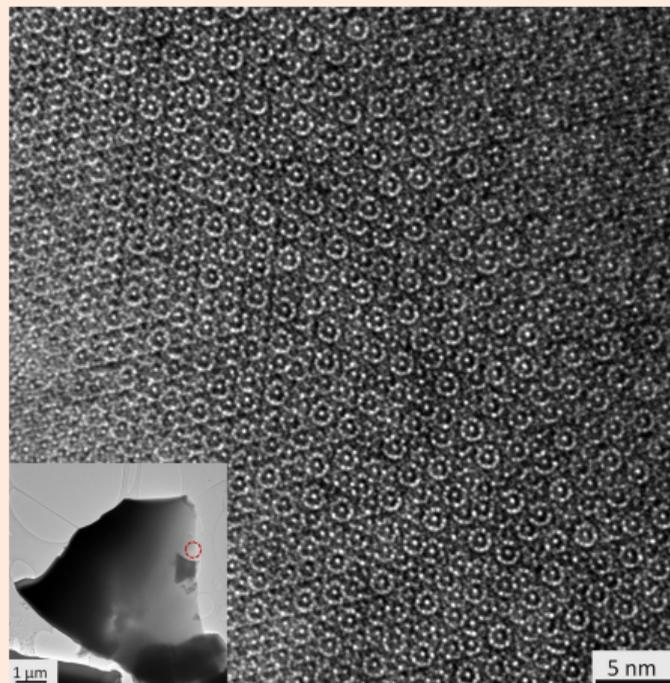
**Figure 1:** HRTEM image of a natural Al<sub>71</sub>Ni<sub>25</sub>Fe<sub>5</sub> Decagonite quasicrystal with plane decagonal rotational symmetry [Bindi et al., 2015, Figure 5].
